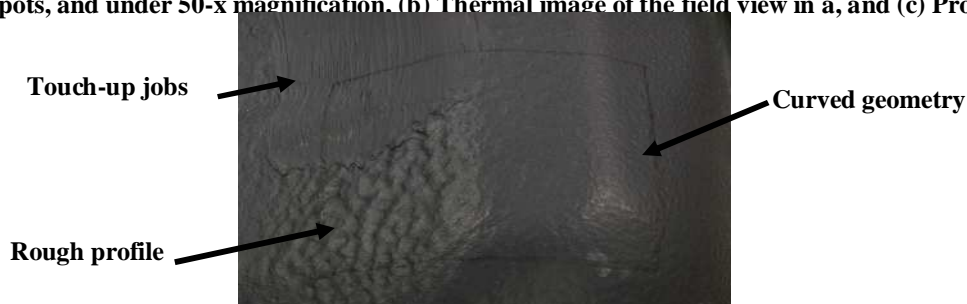
Figure 1. Visual, thermal and post-processed images of an under coated sample container: (a) Visual image for thin spots, and under 50-x magnification. (b) Thermal image of the field view in a, and (c) Processed image
