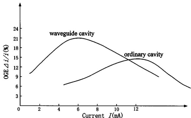
**Fig. 4** OGE as a function of operating current and pressure in an ordinary CO<sub>2</sub> laser: pressure  $P=30$  Torr; waveguide CO<sub>2</sub> laser, pressure  $P=80$  Torr,  $f=1000$  Hz.
