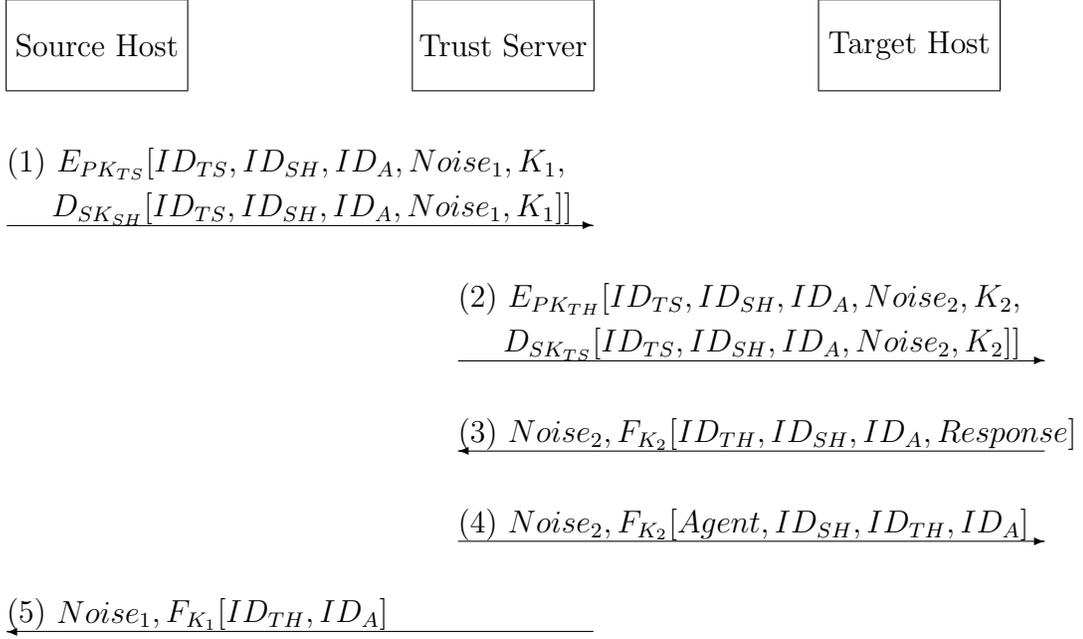
Figure 2: The first secure transportation scheme for the mobile agent
