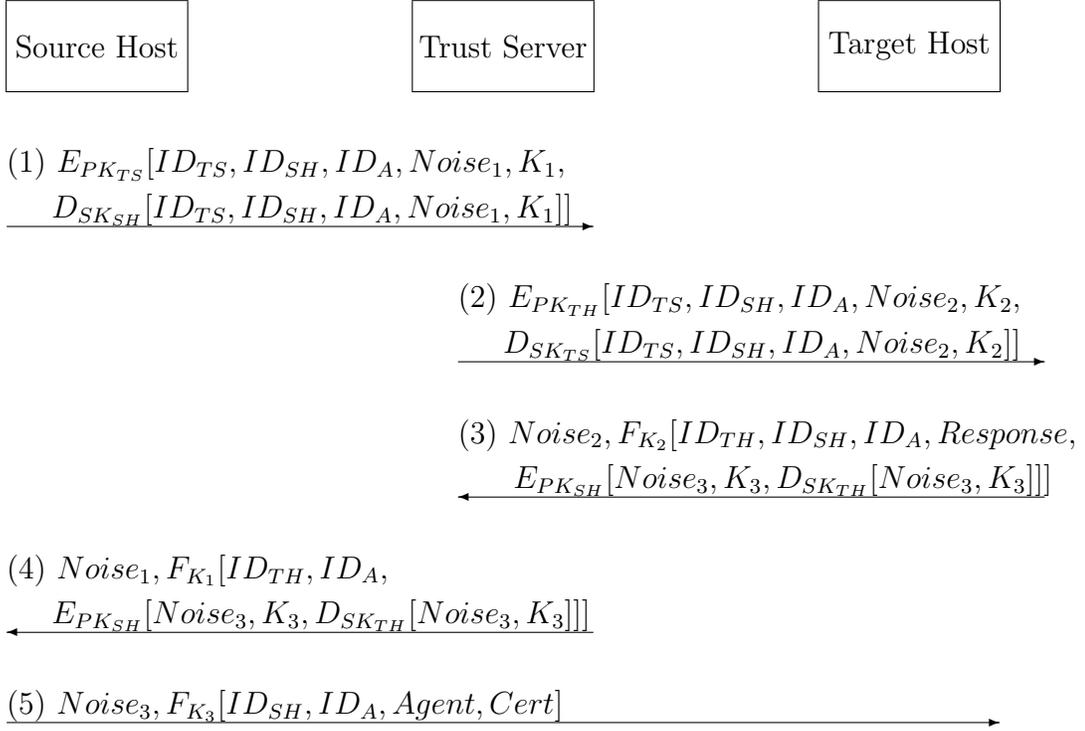
Figure 3: The second secure transportation scheme for the mobile agent
