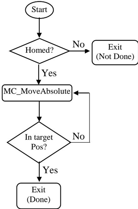
Fig. 4. Experiment motion profile routine flowchart for carriage
