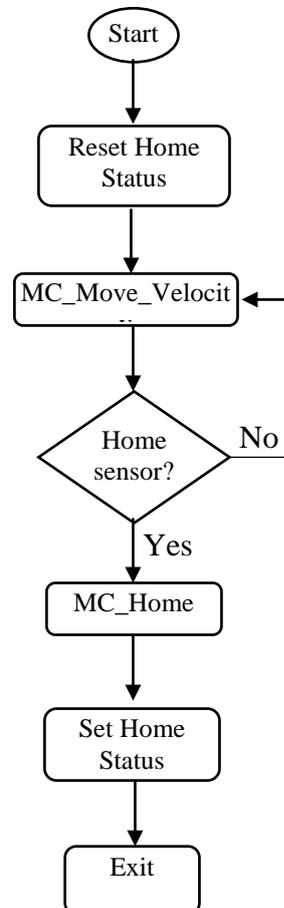
Fig. 3. Homing routine flowchart for carriage
