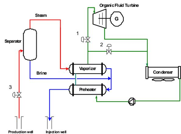
Figure 6: Typical unit process flow diagram
