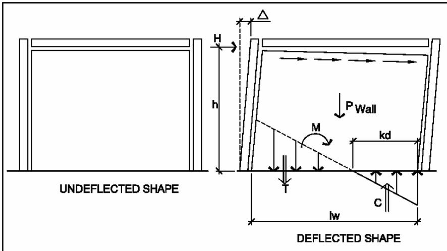
**Figure 5.** Ordinary Hybrid Shear Wall
