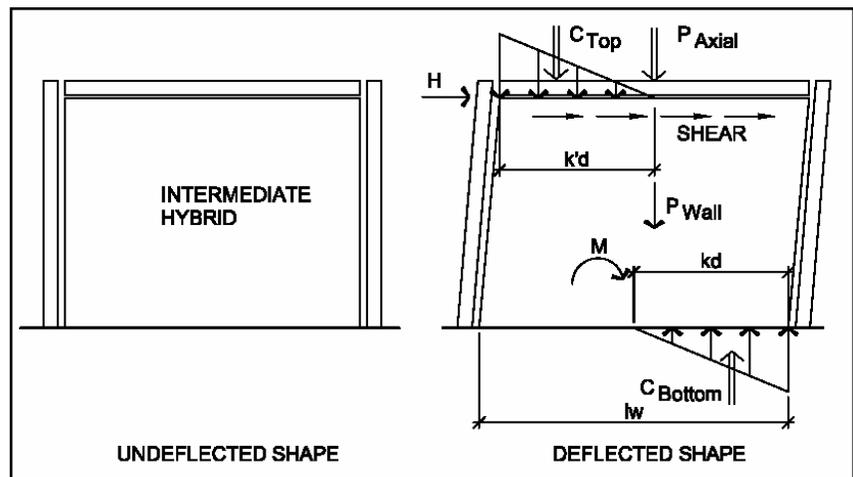
**Figure 6.** Intermediate Hybrid Shear wall
