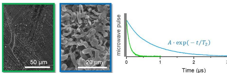
**Figure:** Electron microscopy images of pristine lithium metal anode (green frame) and electrochemically deposited microstructured lithium (blue frame). The lithium metal morphology gives rise to pulse EPR responses with characteristic relaxation times, which can be used to monitor transient morphology changes.
