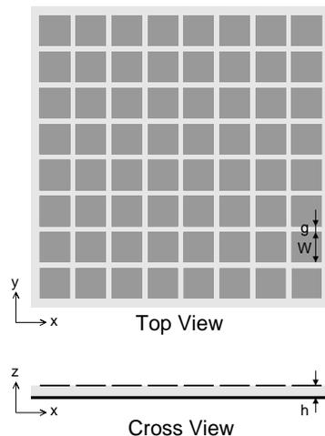
Fig. 1. Geometry of an artificial ground plane: a thin grounded dielectric slab loaded with periodic square patches.
