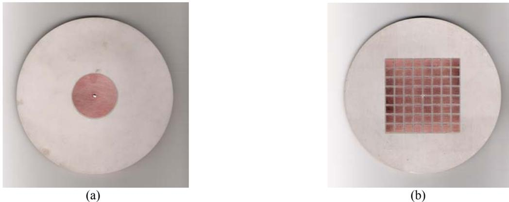
Fig. 3. Photos of a patch fed surface wave antenna: (a) a circular patch in the middle layer with a probe connected to its center, and (b) periodic square patch array on the top layer.
