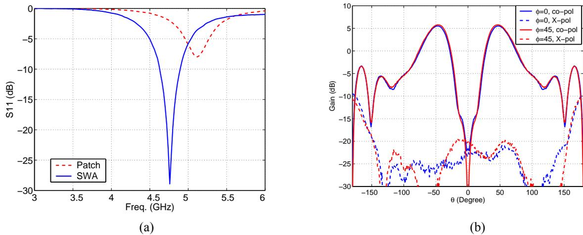
Fig. 4. Radiation performance of the patch fed surface wave antenna: (a) return loss and (b) radiation pattern.
