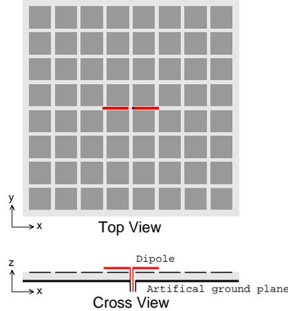
Fig. 2. A horizontal dipole antenna near a patch loaded grounded slab.
