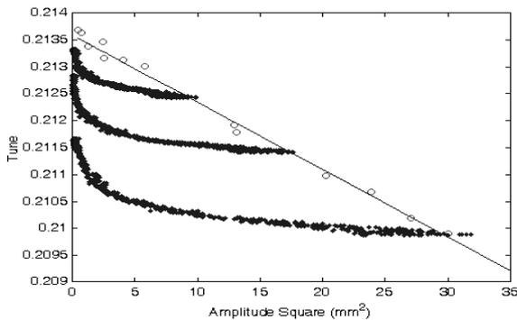
Figure 1: Comparison between the instantaneous tune vs. the square of the amplitude and the tune measured with plain fft method using the whole set of beam position data.
