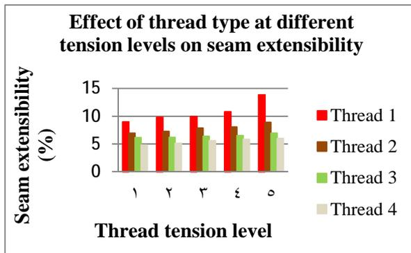
Fig.5. Effect of thread type at different tension levels on seam extensibility
