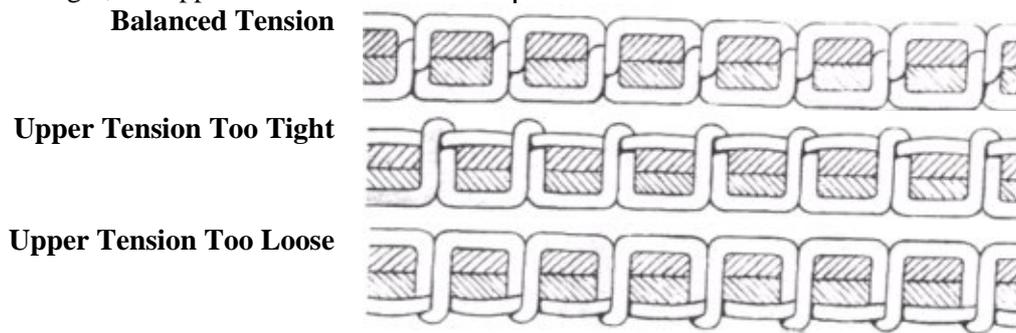
Fig.1. Effect of tension control on sewing stitches. (11)
