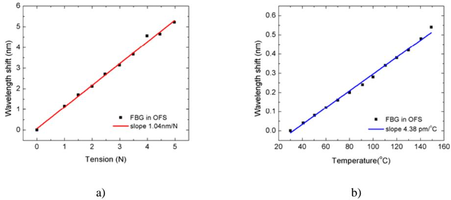
Fig. 3 Dependence of the wavelength shift of the FBG written in OFS fiber on a) applied tension and b) temperature.
