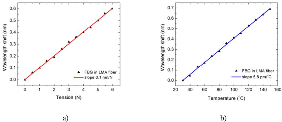
Fig. 4 Dependence of the wavelength shift of the FBG written in LMA fiber on a) applied tension and b) temperature.
