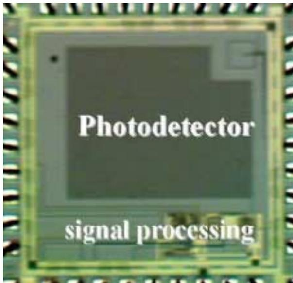
Fig. 2. The microluminometer integrated circuit.
