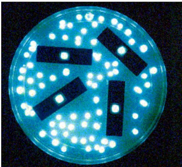
Fig. 1. This photograph shows maximally-induced bioluminescent bacteria on a CMOS microluminometer to form bioluminescent bioreporter integrated circuits. All the light for this photograph was provided by the bacteria (45 minute exposure time).
