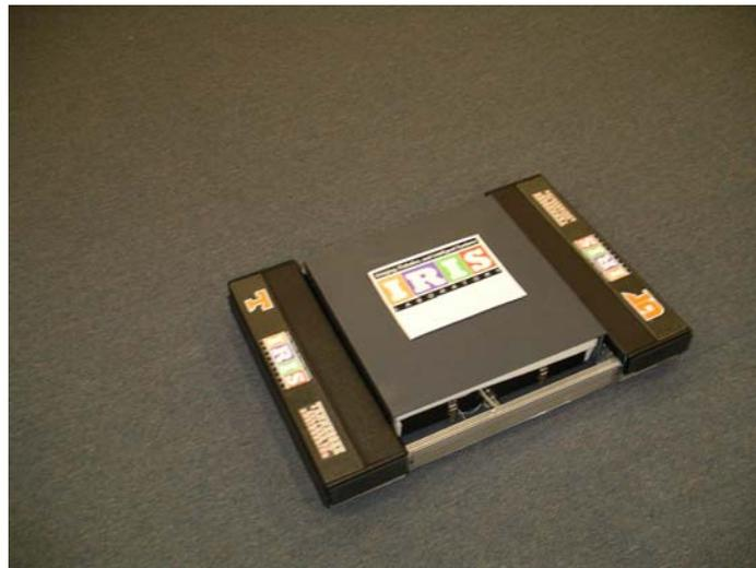
Fig 2. Track driven Safobot robot with the radiation sensor mounted in the center.
