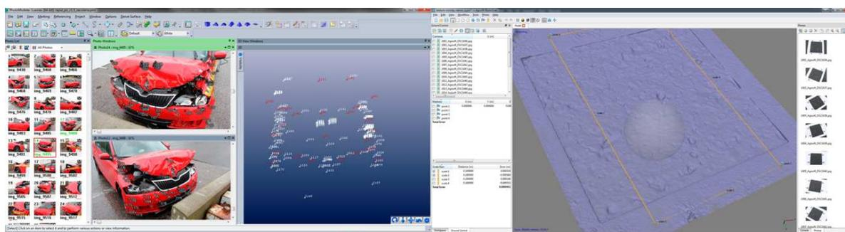
Figure 1: Vehicle deformation measurements in PhotoModeler Scanner and a road pavement model in Agisoft PhotoScan
