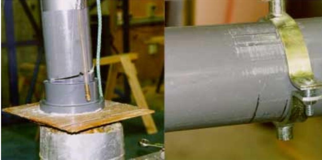
**Figure 6 Fractured pipe at flange (flange disconnected) and evidence of support bracket movement on pipe**
