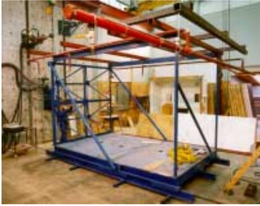
**Figure 4 Sprinkler system on shake table**
