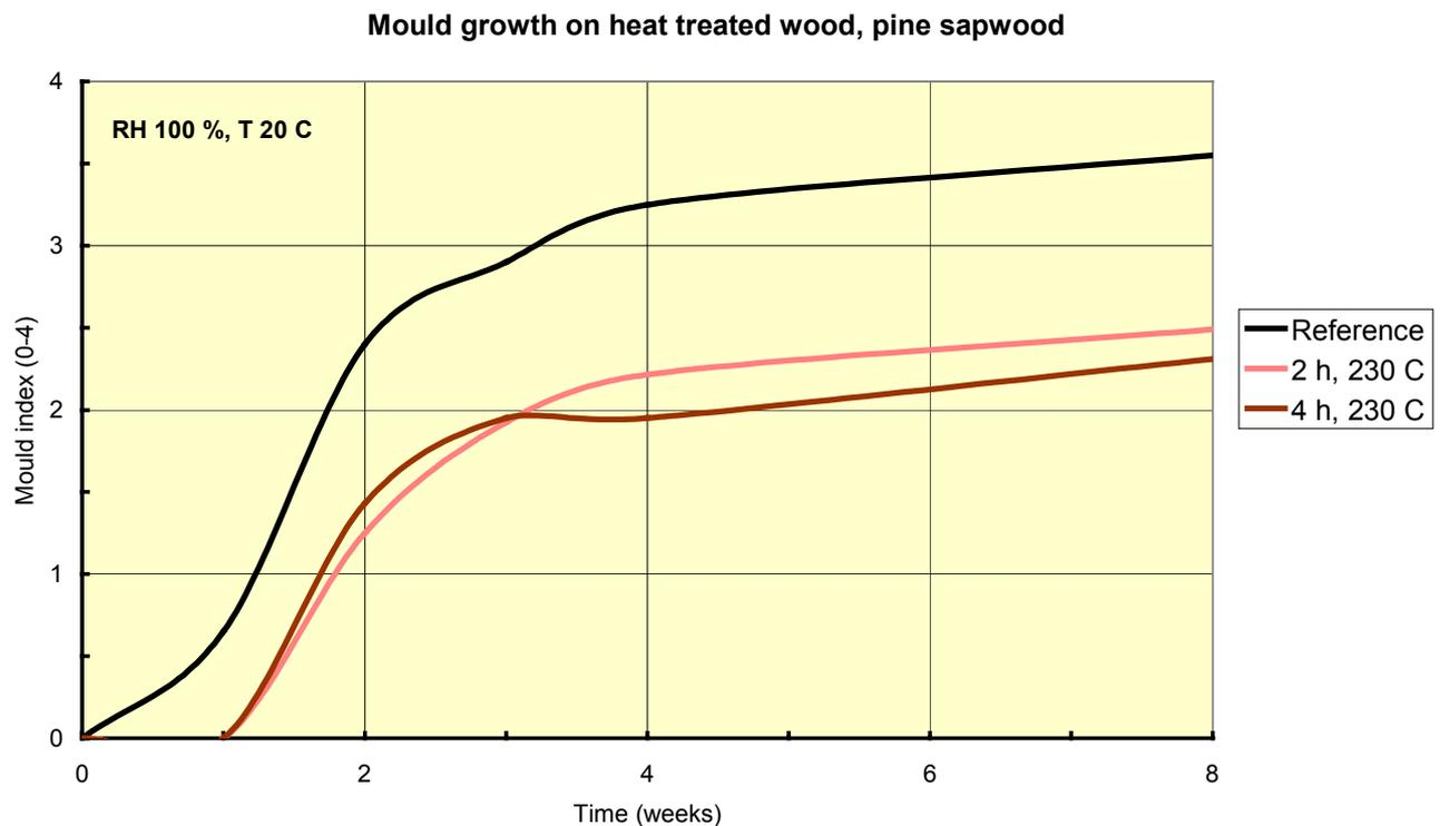
**Figure 2.** Mould growth at 100% RH and 20 °C during 8 weeks.
