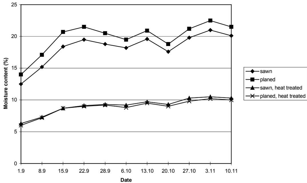
**Figure 1.** Moisture content of the spruce panels painted with the water-borne acrylic paint 1994.
